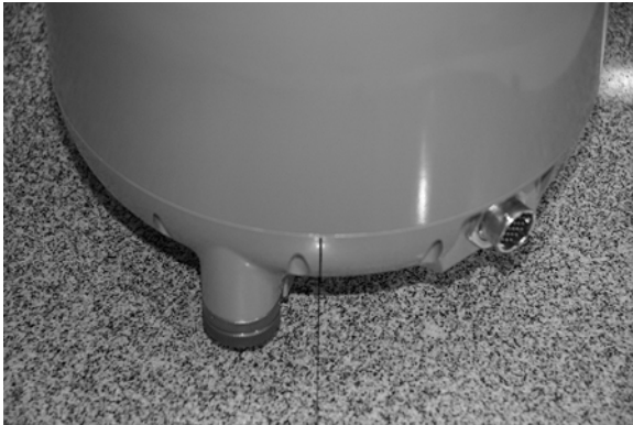
Figure 3-1 Example of seismometer alignment using vertically scribed marks
