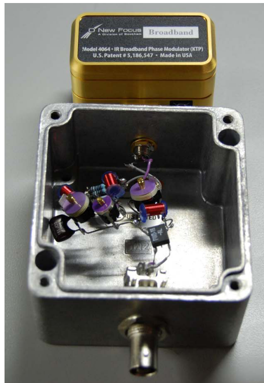
Figure 12: Picture of flying-component circuit in box attached to EOM
