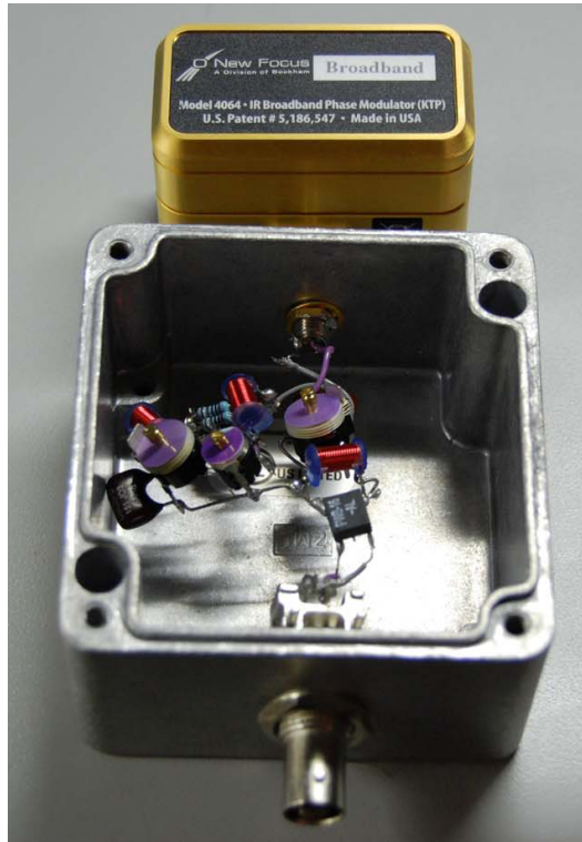
Figure 17: Picture of flying-component circuit in box attached to EOM
