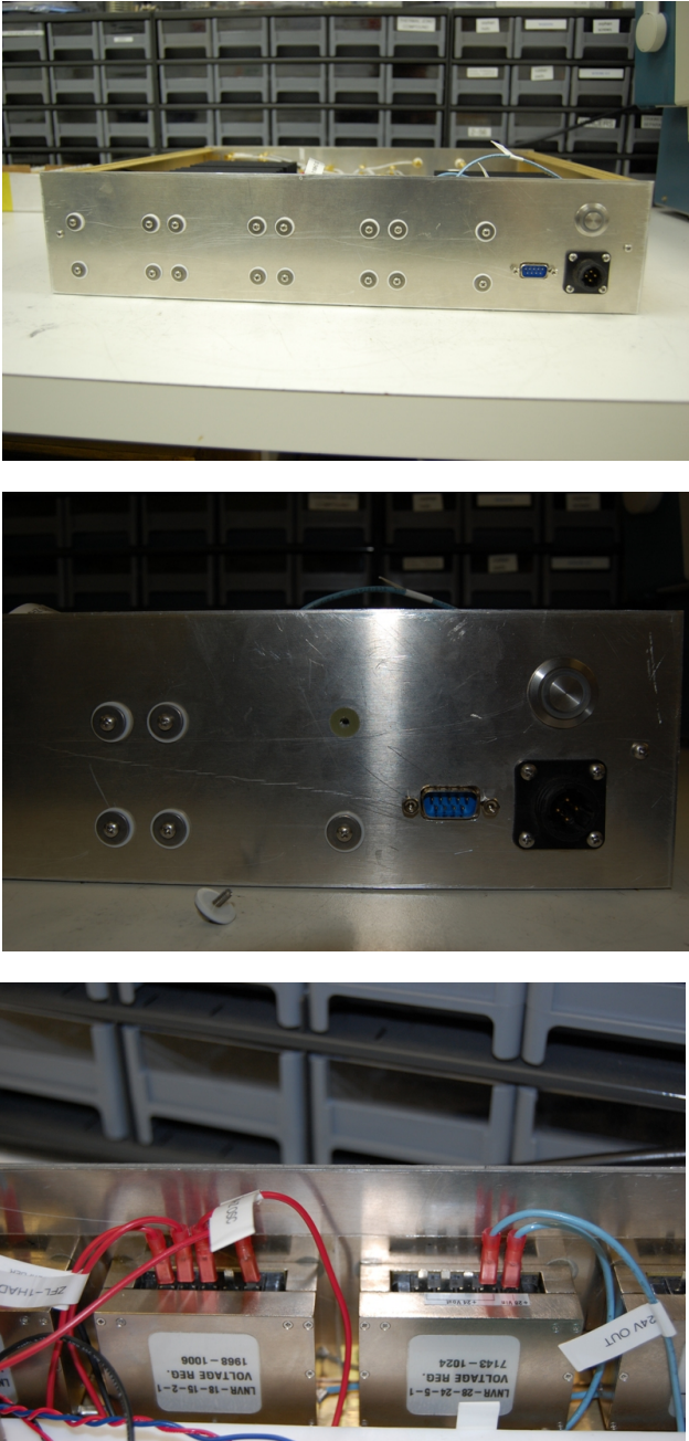
Figure 5: LNVRs attached to the back panel. Electrical isolation is guaranteed by MICA sheets, G10 through-hole rings, Teflon washers.
